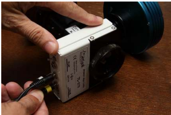
FIGURE 2.5 – Connect the yellow connector to the Alpy calibration lamp
