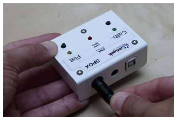
FIGURE 2.2 – Connect the 4 pins cable
