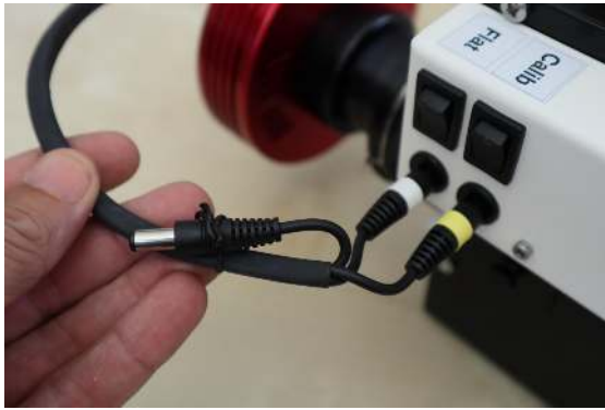
FIGURE 2.12 – Attach the unplugged connector
