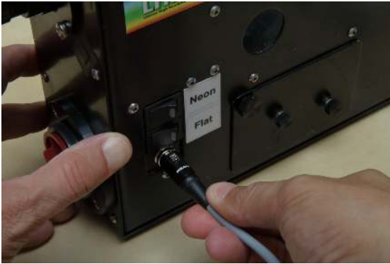
FIGURE 2.9 – Connect the cable to the Lhires III
