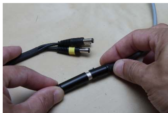
FIGURE 2.3 – Connect the 4 pins cable to the Alpy adapter cable
