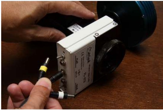
FIGURE 2.4 – Connect the black connector to the Alpy center pin
