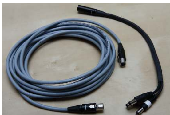
FIGURE 1.2 – 4 pins cable and Alpy / LISA adapter cable (right)
