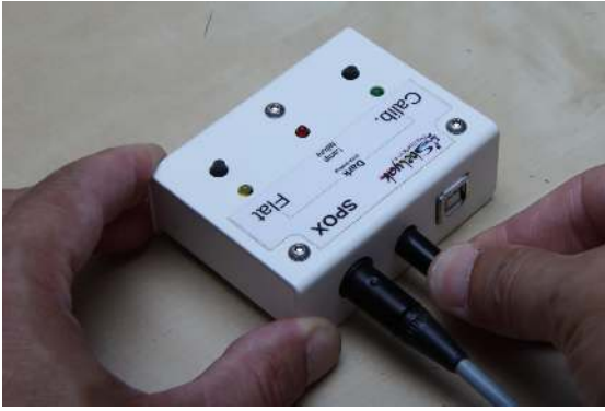
FIGURE 2.8 – Connect the power supply to SPOX
